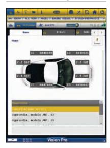
Based on the data read by TPMS Connect EVO\*, it is easy to encode the TPMS control unit with new sensors.
