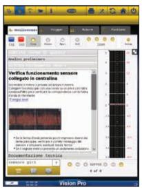
Helpful guide on operating the oscilloscope with the function of pre-selecting the measurement scale and relevant charts related to the testing of electrical components of the vehicle such as sensors, actuators, etc.
